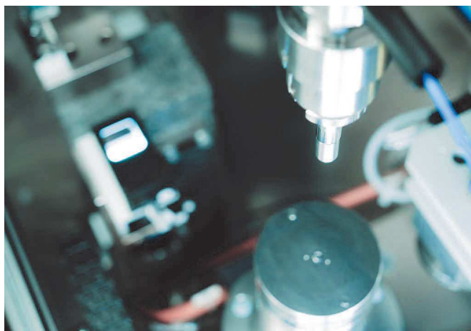
Station de chassage.
